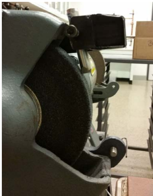
Figure 5: Steel sample held against grinding wheel by swing arm.
